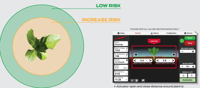
Actuator open and close distance around plant is based on center of the plant
