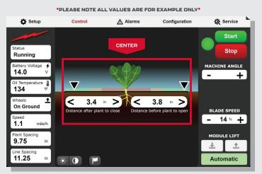
Actuator open and close distance around plant is based on center of the plant
